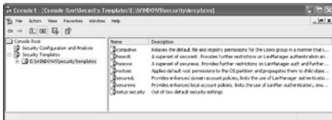
Figure 8.4: The Security Configuration Editor provides a number of standard templates for creating your security setup.
