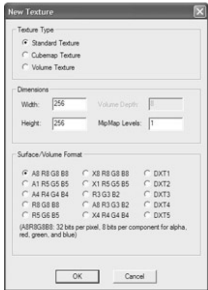
Figure 15.15: The DirectX Texture Tool defines images by texture type, size, and color depth.
