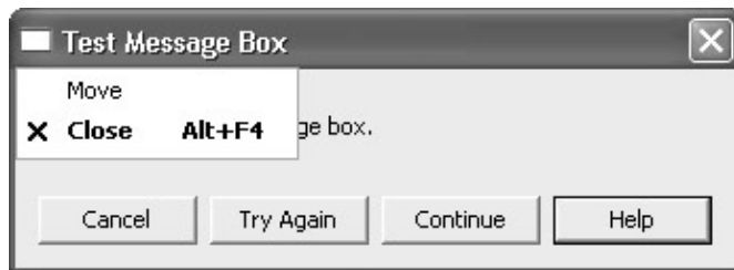
Figure 2.2: The MessageBoxEx() function enables you to add a System menu to your message box.
