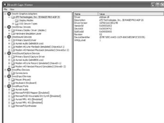
Figure 14.2: The DirectX Caps Viewer tool helps you learn about the DirectX capabilities of your system.
