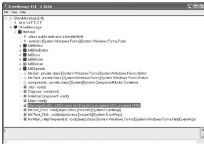
Figure 3.7: To see the imported functions for a managed application, you must view the application in ILDASM.
