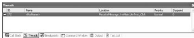
Figure 4.8: The Threads window can be helpful in diagnosing problems with a Win32 API message handler.
