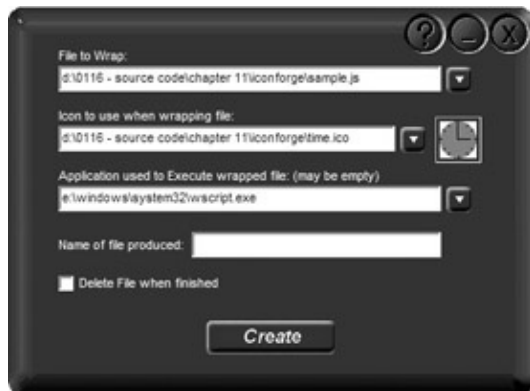
Figure 11.12: The IconWrapper utility enables you to add an icon to a file that doesn't normally accept an icon.
