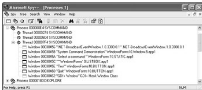
Figure 4.5: Every visible control in an application is very likely a window as well.
