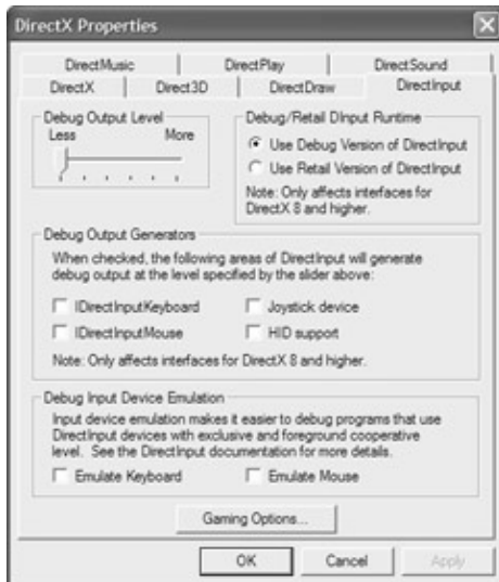
Figure 15.3: The DirectInput tab provides options for controlling which devices generate debug information.
