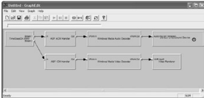
Figure 16.2: Many media files contain two or more data streams, each of which requires separate processing.
