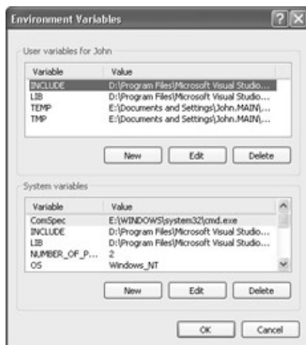
Figure 6.4: The Environmental Variables dialog box contains a set of system and user strings.
