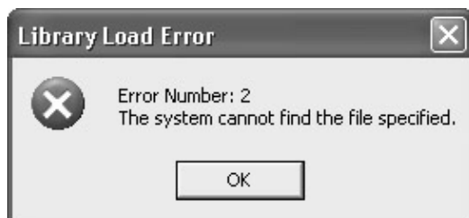
Figure 3.3: An example of a system error message retrieved using FormatMessage()
